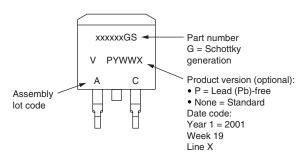
Example: This is a xxxxxxGS with assembly lot code AC, assembled on WW 19, 2001 in the assembly line "X"
